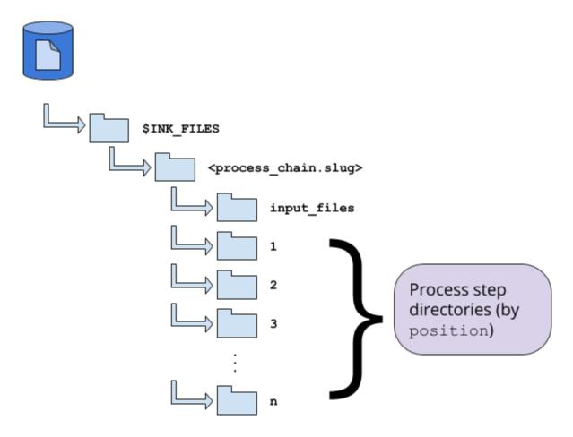
Once the file structure is ready, the files provided by the user are placed into **input\_files**. Before each Step Class executes, INK copies the files from the previous step directory (or **input\_files** if it's the first) and the Step Class runs its code against the files in its directory.
